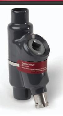
These Plasti-Bond REDH<sub>2</sub>OT sealing fittings should be used with a suitable system of sealing compound, such as Chico A, Chico X or Chico A-P from Crouse-Hinds. Chico Speed Seal may be used on EYS or EYD sizes 1/2" - 2". Follow the installation instructions included with the sealing compound and properly tag after installation to ensure correct classification ratings.
