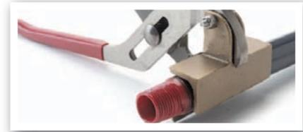
**Z-Wrench** features extra wide jaws which spread the clamping force, enabling the tool to grip without marring the surface of the conduit. The "V" shaped upper jaw allows **Z-Wrench** to accommodate a wide range of conduit sizes. Shallow grooves in the upper and lower jaws provide an excellent grip.
