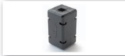
**Plasti-Socket** is a fiber-glass encapsulated 3/8" drive socket for use with the square fiberglass encapsulated U bolt and beam clamp nuts used in the Plasti-Bond RED-H<sub>2</sub>OT conduit support system. The **Plasti-Socket** helps avoid coating damage from metal sockets, pliers or wrenches.
