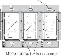
Middle of ganged switches/dimmers have all fins removed
