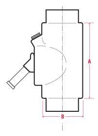
EYDX - EXPANDED FILL FEMALE HUBS WITH DRAIN. FOR SEALING IN VERTICAL POSITIONS ONLY.
