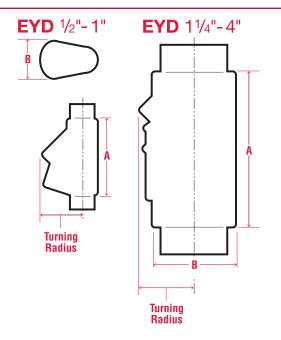
EYD - FEMALE HUBS WITH DRAIN. FOR SEALING IN VERTICAL POSITIONS ONLY.
