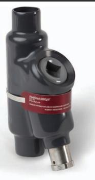
These Plasti-Bond REDH<sub>2</sub>OT sealing fittings should be used with a suitable system of sealing compound, such as Chico A, Chico X or Chico A-P from Crouse-Hinds. Chico Speed Seal may be used on EYS or EYD sizes 1/2" - 2". Follow the installation instructions included with the sealing compound and properly tag after installation to ensure correct classification ratings.
