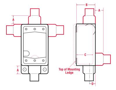
All configurations offered in both 'FS' or 'FD' box depths. FS prefix: Shallow configuration, FD prefix: Deep configuration
