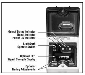
Figure 1. Indicators and controls on the Q45VR3 Series Sensors
