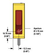
Figure 12. Laser Aperture Location
