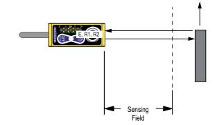
A reflective background object in this position or moving across the sensor face in this axis is ignored.
