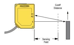
A reflective background object in this position or moving across the sensor face in this axis and direction may cause a false sensor response.
