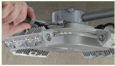
**Step 3** Lift and slide fixture until it clicks. Lock release tabs with captive hardware. Aim and lock optical panels.
