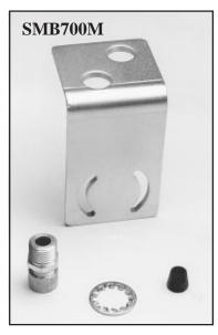
Heavy-duty 1/4-inch (6mm) zinc plated steel bracket that allows the MAXI-BEAM to retrofit to installations of MICRO-SWITCH models MLS8 or MLS9 sensors. Includes cable gland and lockwasher.
