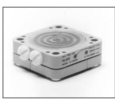
MAXI-BEAM sensors offer built-in timing logic with the addition of a logic module. There are two logic modules available. Model RLM5 is programmable for ON-DELAY, OFF-DELAY, and ON/OFF DELAY timing logic. Model RLM8 offers both ONE-SHOT and DELAYED ONE-SHOT functions. A programming ring is supplied with each logic module. Programming of the logic function, timing range, and output state is similar to sensor head programming.
