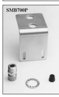
Heavy duty 1/4-inch (6mm) zinc plated steel bracket that allows the MAXI-BEAM to retrofit to installations of PHOTOSWITCH series 42RLU and 42RLP sensors. Includes cable gland and lockwasher.
