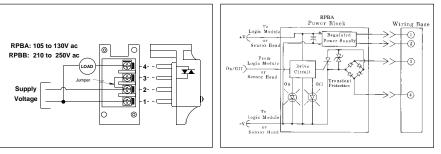
Power block models RPBA and RPBB are the most commonly used for ac MAXI-BEAM operation. As the typical hookup shows, they are intended to switch the same ac voltage as is used to power the MAXI-BEAM. However, both can switch any ac voltage that is lower than the supply voltage, as long as both ac circuits share a common neutral. Observe local codes whenever mixing ac voltages in a common wiring chamber.
