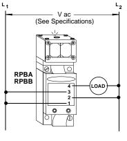
CAUTION: the output switch will be destroyed if the load is shorted.
