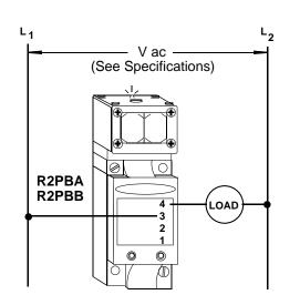
MAXI-BEAM sensors using power block R2PBA or R2PBB wire in series with an appropriate load. This combination, in turn, wires directly across the ac line. A 2-wire sensor may be connected exactly like a mechanical limit switch.
