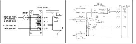
Model RPBR operates the MAXI-BEAM with either ac or dc. It offers an SPST "hard" relay contact between wiring base terminals #3 & #4, which allows the MAXI-BEAM sensor to directly interface with loads which draw high current. It also allows series connection ("AND" logic) with multiple dc sensors.
