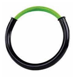
The 4.5mm 240' SIMpull<sup>TM</sup> Fish Tape Tube is designed to offer superior performance on long runs. With the same features and benefits as previous models, the fish tape tube is designed for longer runs of up to 240 feet. It also includes both a glow-in-the-dark, non-conductive leader and a flexible metal leader on opposite ends, allowing for usage in both empty and filled conduit.
