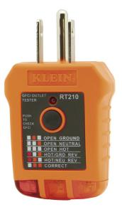
Klein Tools Receptacle Testers are designed to detect the most common wiring problems in standard and GFCI receptacles. A convenient chart on the tester helps determine wiring condition in outlet, based on lights results. Conditions indicated: open ground, reverse polarity, open hot, open neutral, hot/ground reversed.
