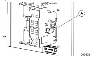
Figure 3-4. Auxiliary Contact
