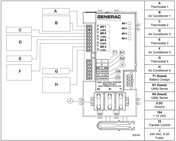
Figure 3-3. Typical SACM Connections
