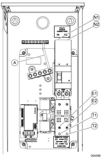
Figure 3-2. Wiring Connections
