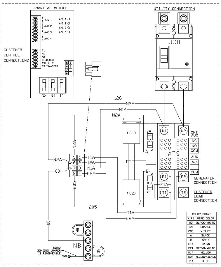
WIRING - DIAGRAM SE TRANSFER SWITCH 100-200A DRAWING #: 10000006038
