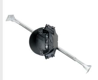
4" Round Ceiling Box with a bar hanger that adjusts to 16" or 24" joist spacing. It has four Auto/Clamps. It is constructed with impact-resisitant Noryl thermoplastic, making it virtually unbreakable and non-conductive. Its depth-mounting gauge at bottom of bracket helps you align the box at the proper depth relative to the ceiling. 50 pack.
