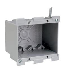
Double Gang, Old Work Switch and Outlet box with swing-bracket for mounting, adjusts from 1 1/4" to 1/8". It has four Auto/Clamps for each end. It has a durable, impact-resistant thermoplastic box. The metal swing bracket is for quick mounting in existing walls. 50 pack.
