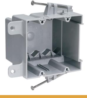
Double Gang Switch and Outlet Box with captive mounting nails on each end and four auto alamps on each end. It is easy to install with a rectangular cutout. It is durable and has an impact-resistant thermoplastic box. It contains innovative extras that cut installation time. 50 pack
