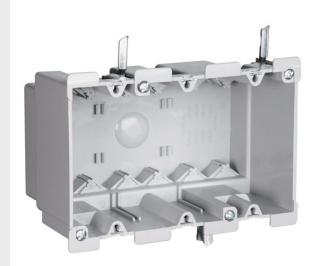
Triple Gang, Old Work Switch and Outlet Box with Swing-Bracket for mounting. Adjusts from 1 1/4" down to 1/8". Six Auto/Clamps for Each End. 10 pack.
