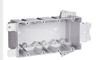
Four Gang, Wood and Steel Stud Bracket Box with Quick/Click. 3/8" offset for wood and steel stud mounting. Rear stabilizing bar virtually eliminates inward movement. Six Auto/Clamps at each end. For use with 3/8" to 5/8" wallboard. 25 pack.
