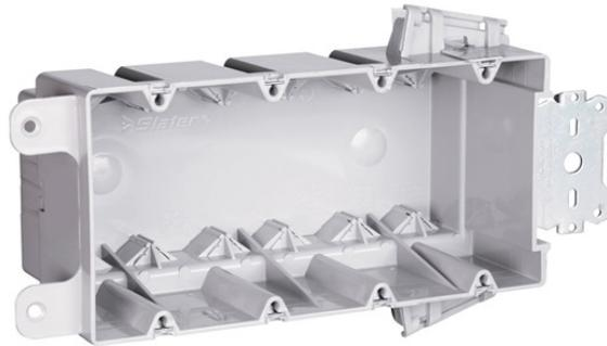
Four Gang, Wood and Steel Stud Bracket Box with Quick/Click. 3/8" offset for wood and steel stud mounting. Rear stabilizing bar virtually eliminates inward movement. Six Auto/Clamps at each end. For use with 3/8" to 5/8" wallboard. 25 pack.
