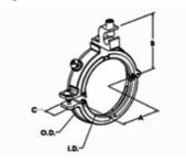
Dimension A in Inches: 1.37 Dimension B in Inches: 1.90 Dimension C in Inches: 0.73 Dimension D in Inches: 1.02 Dimension E in Inches: 1.80
