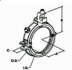
**Download Photo Image** Dimension A in Inches: 1.67 Dimension B in Inches: 2.08 Dimension C in Inches: 0.73 Dimension D in Inches: 1.55 Dimension E in Inches: 2.30
