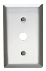
Single gang, Single telephone or cable outlet removable 13/32" ID grommet in 17/32" hole. Strap mounted with adjustable yoke. One #340 yoke. 302 Smooth stainless steel.
