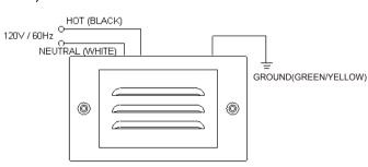
2) Insert Fixture into the Wall Single-Gang Box. Secured with mounting screws(2).
