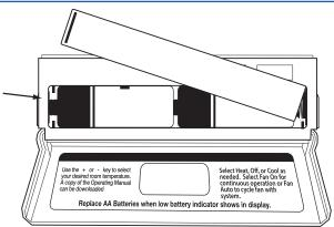
Insert 2 AA Alkaline batteries (included). High quality Alkaline batteries are recommeded.
