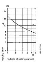
Tripping curve of overload relay T .. starting from cold state
