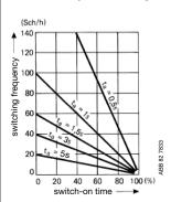
Switching frequency depending on duty ratio ED in %, ta: Motor starting time
