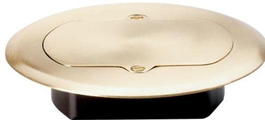
Low-Profile Brass Cover requires minimum 3/8" hardwood floor thickness. Includes 885 15 amp, 125 volt Decorator Duplex receptacle and will accept any decorator device. Cover includes captive screws to prevent loss.
