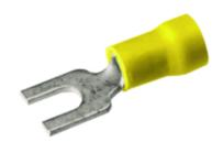
Insulated Brazed Fork Terminal, Insulated Brazed Fork Terminal, Smooth Entry, #12-#10, 600V, #6-#8 Stud, Vinyl Insulated, Tin Plated.
