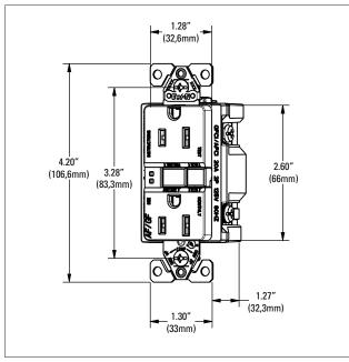
Figure 1. OBC TRAFGF 15A Line art with dimensions
