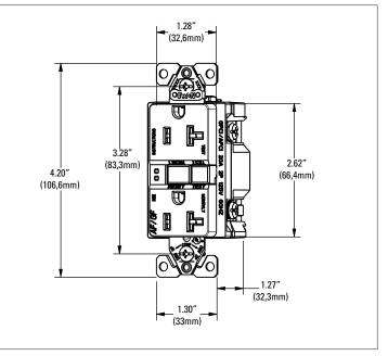
Figure 2. OBC TRAFGF 20A Line art with dimensions
