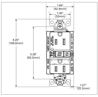
Figure 1. TRSGFNL15 Line art with dimensions
