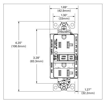
Figure 2. TRSGFNL20 Line art with dimensions
