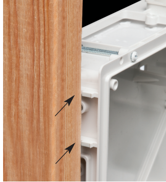
Positioning tabs are set for 1/2" or 5/8" drywall.
