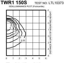
W lamp, horizontal lamp orientation Footcandle values based on 12' mounting height, 15800 rated lumens. Luminaire Efficiency: 54.6%
