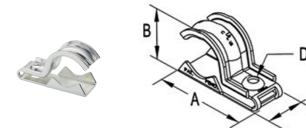
The one piece clamp back and strap secures both cable and conduit. The UCS-5075 secures 1/2" and 3/4" EMT, Rigid, IMC, PVC/Polyolefin Coated Rigid, PVC/Polyolefin DIA Soated IMC, Metallic Liquid Tight, Nonmetallic Liquid Tight, FMC, and Schedule 40 and Schedule 80 PVC conduit, as well as .710" 0 to 1.10" 0 steel and aluminum AC/MC cable. Plenum Rated for use in Air Handling systems, per UL 2043.
