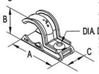
Dimension A in Inches: 4.20 Dimension B in Inches: 2.96 Dimension C in Inches: 1.20 Dimension D in Inches: 0.34
