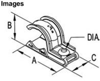
Download Photo Image Dow Dimension A in Inches: 2.42 Dimension B in Inches: 1.47 Dimension C in Inches: .970 Dimension D in Inches: .255
