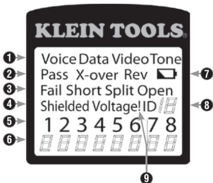
1. **Mode:** The top line of the display shows the cable type test mode or tone generation mode.
