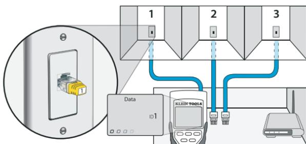
1. **Insert a numbered LanMap™ Location ID Remote into the RJ45 port** of each room that needs to be identified. Write down pairs of numbers and room names for later.
