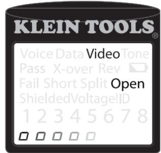
**Coax Cable with an Open:** There is a break in the cable continuity. A break in the shield or in the center wire can cause an open fault. The cable does not pass and the ID remote number on the other end of the cable cannot be determined.
