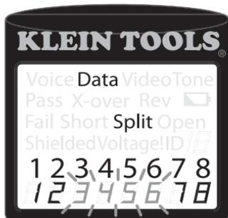
**T568A Cable with Split Pairs:** A common error in building a cable is to put all the pairs in pin sequence 1-2, 3-4, 5-6 and 7-8. This will produce the correct continuity, but the pairs are designated to be on pins 3-6 and 4-5 in the middle of the connector for compatibility with phone wiring. This wiring error is only detected by the split pair test since the designated pairs are not twisted together.
