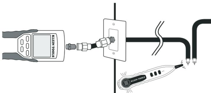
1. **Attach barrel connector** to the open coax port on the top of the main tester body.
