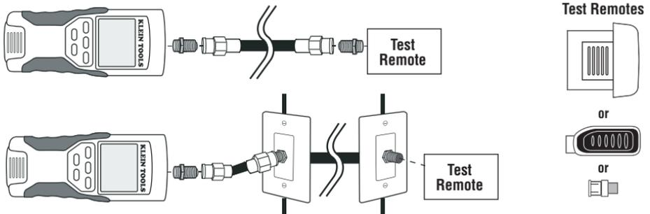
1. **Attach barrel connector** to the open coax port on the top of the main tester body.
