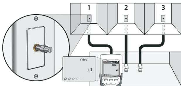
1. **Insert a numbered CoaxMap™ Location ID Remote into the F-connector port** of each room that needs to be identified. Write down pairs of numbers and room names for later.
