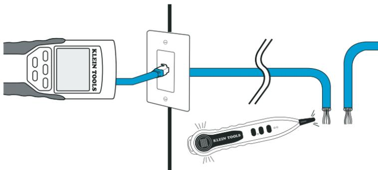
1. **Connect a known working patch cable** to the RJ45 port (if you are tracing an Ethernet cable) or RJ12 port (if you are tracing a phone cable) located at the top of the main tester body.
