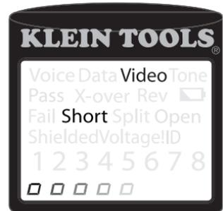
**Coax Cable with a Short:** The center wire of the cable is connected to the shield, creating a short. The cable does not pass and the ID remote number on the other end of the cable cannot be determined.
