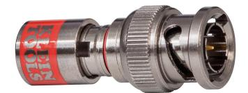
Klein's patented universal sleeve technology BNC connectors install up to 2x faster than other BNC compression connectors. Patented viewing windows in sleeve aid in proper seating. One connector fits all diameter variations within a cable series. This patented sleeve design provides the excellent holding power and signal strength you demand.
