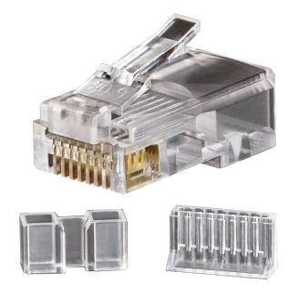
Klein's data and telephone plugs are professional-grade and deliver consistent, reliable performance. Our thick 50 micro-Inch gold plating on contacts prevent erosion and extended connector life. The three-pronged contacts provide more reliable connections with solid and stranded wire. The plug is housed in a durable resin with a spring clip. Expect a sure connection each and every time.
