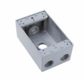
Weatherproof 1 Gang Box, 4 Hole 1/2", 18.0 Cu.In., Gray (2 Holes One End, 1 Hole Other End, 1 Hole in Back)
