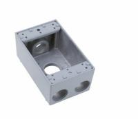
Weatherproof 1 Gang Box, 4 Hole 3/4", 18.0 Cu.In., Gray (2 Holes One End, 1 Hole Other End, 1 Hole in Back)
