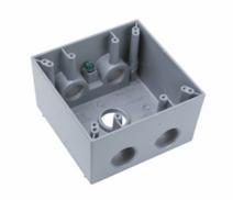
Weatherproof 2 Gang Deep Box, 5 Hole 1/2", 37 Cu.In. with Threaded Holes, Gray (2 Holes Each End, 1 Hole in Back)
