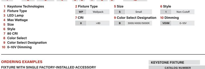
FIXTURE WITH SINGLE FACTORY-INSTALLED ACCESSORY KT-WPLED20-S1-8CSB-VDIM /515P6
