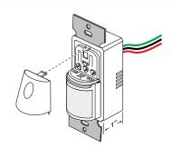
Extremely shallow (1") back housing and 6" flying leads facilitate quick installation in standard wall box
