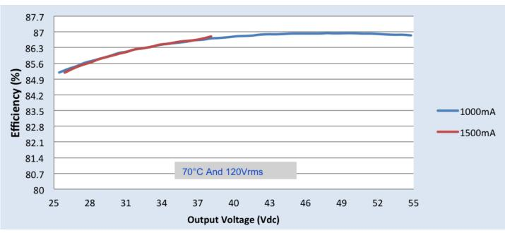
Efficiency Vs. Output Voltage at 277Vac
