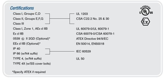
NOTE: Where reference is made to Class I and Class II hazardous locations, the equipment is suitable for both Division1 and Division 2 locations.
