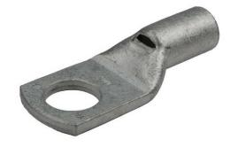
Copper Compression Lug, Ring Tongue, 1 Hole w/ Inspection Hole, AN-3/0 Flex, 3/8" Stud, Short Barrel, Tin Plated.
