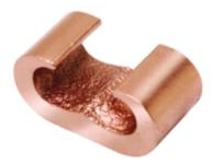
Copper Compression C Connector, 1 - 2/0 AWG(Str), 3/8" Rod (Run) & 1 - 2/0 AWG(Str) (Tap).
